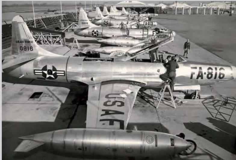
A line-up of Lockheed F-94B-1-LO Starfires. The F-94 was an interim all-weather fighter produced from the T-33 trainer to fill the gap left by the delayed Northrop F-89 programme. 854 aircraft were built in three versions and they saw service with the USAF and Air National Guard from 1950 to 1959.
